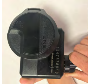
Figure 22 – Connecting the Coaxial Cable
