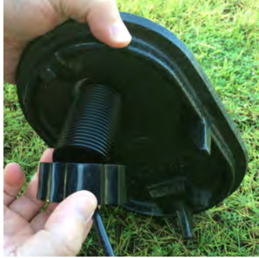
Figure 17 – Locking the Nut on the Antenna
