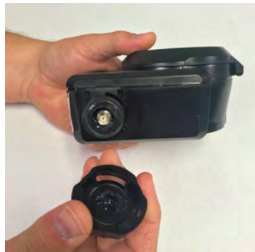
Figure 20 – Removing the Dust Cover
