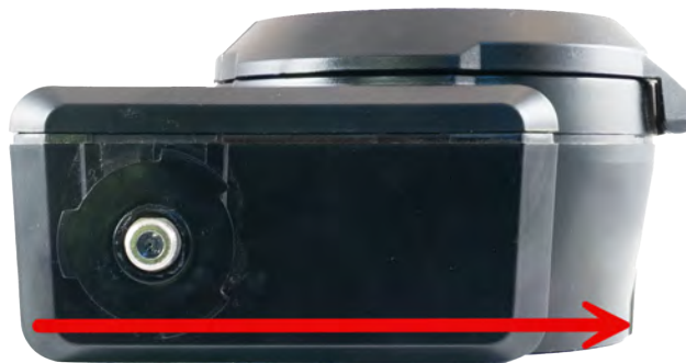
Figure 23 – Cellular ProCoder™)R900i™ with Arrow Showing Direction of Magnet
