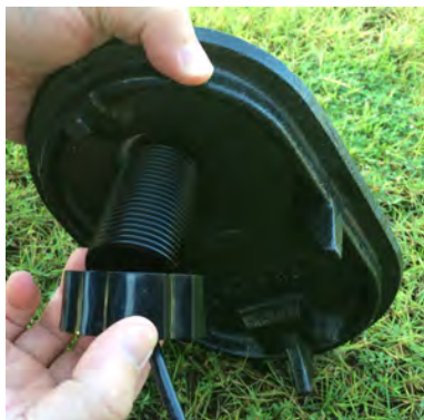
Figure 24 – Locking the Nut on the Antenna
