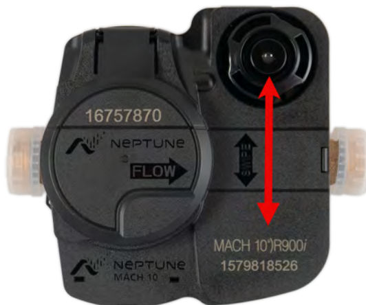
Figure 30 – MACH 10® R900i™ with Arrow Showing Direction of Magnet Swipe
