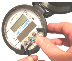
Figure 4: Routing the Wire
