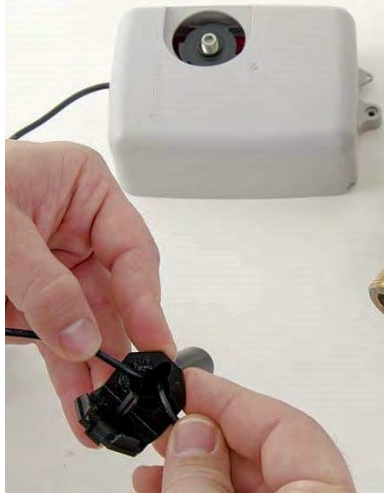
Figure 17 – Gray Wires in Slot
